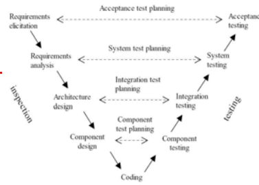
Figure 1. V-model of software testing
